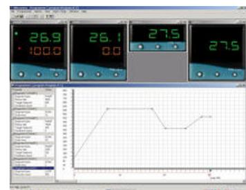
The instrument is mounted on machines or other measurement position at the "factory site" where the machine operator can see process values or set point values and can directly via the buttons set another set point value or another configuration.
